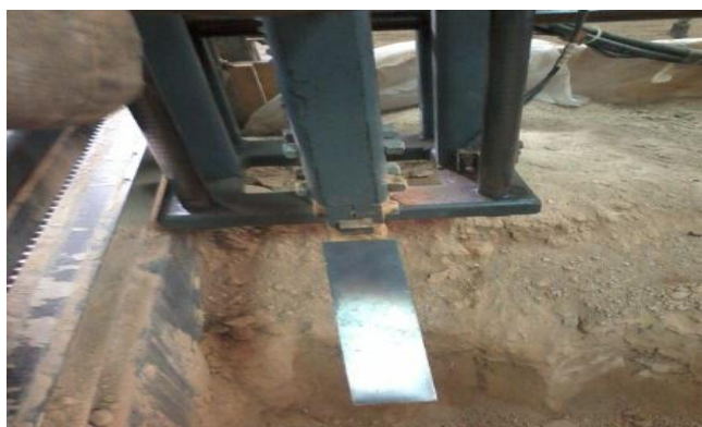
Figure 2: A simple tillage tool used in the soil bin experiments
