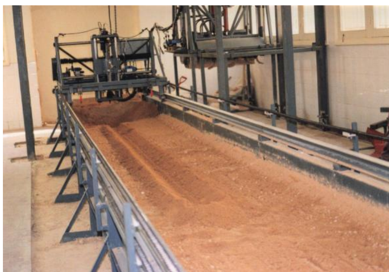
Figure 1: Soil bin facility
